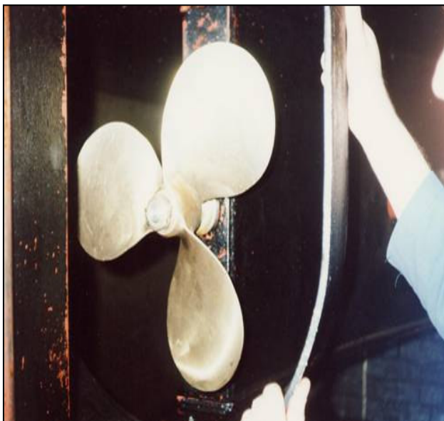
Figure 20.1. Fitting a propeller shroud
