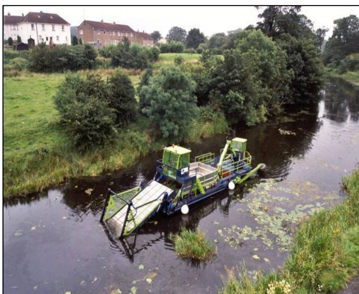
Figure 16.1. Boat mounted vegetation control (Berkenheger weed boat)
